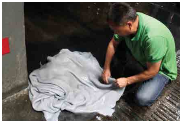
Figure 2. Inspection of delimed and bated hides. Time saved within the processing allows optimum time in deliming/washings for the maximum removal of Inorganic salts, solubilized proteins and fats from deep within the fiber structure.
